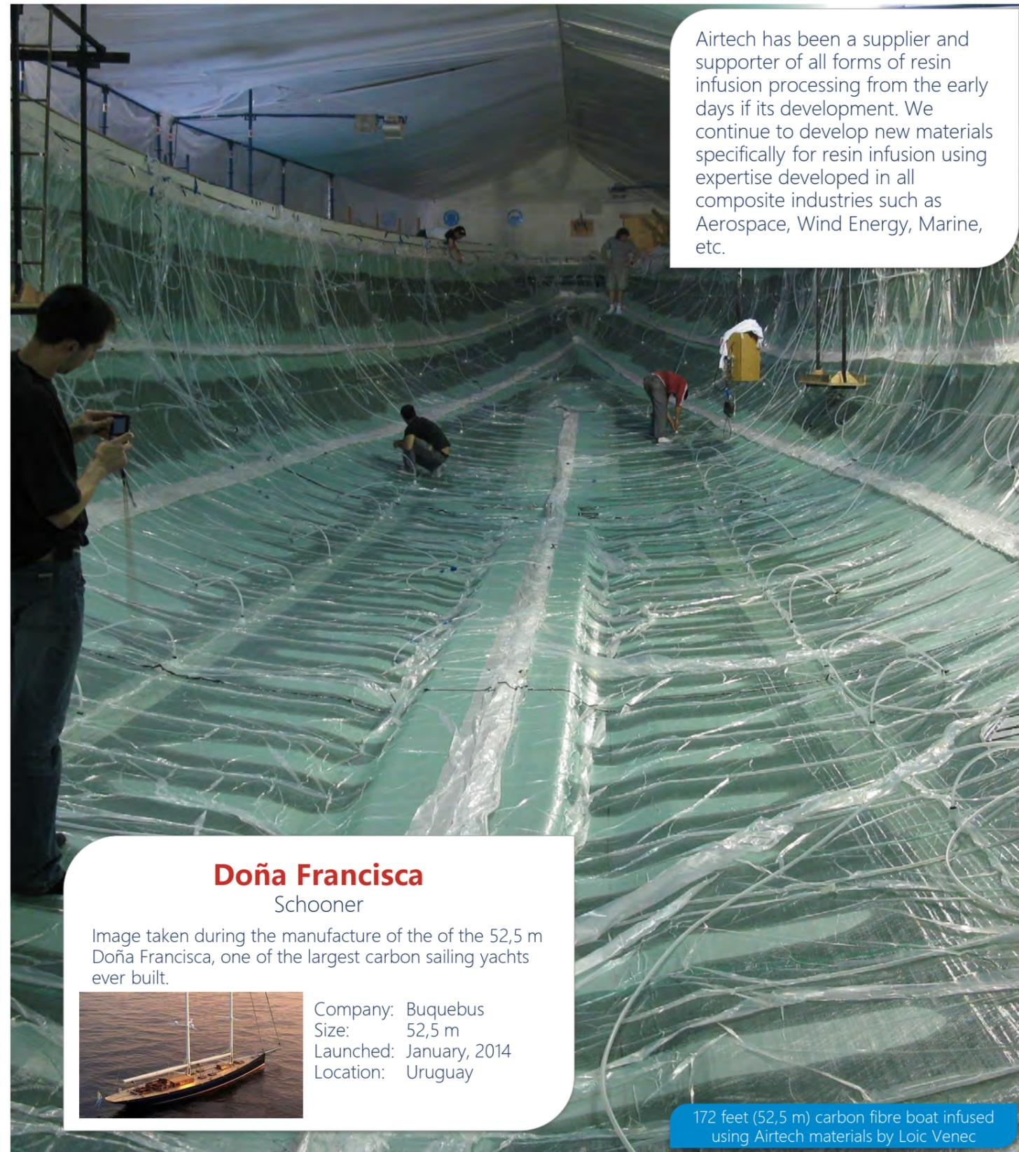
Airtech has been a supplier and supporter of all forms of resin infusion processing from the early days of its development. We continue to develop new materials specifically for resin infusion using expertise developed in all composite industries such as Aerospace, Wind Energy, Marine, etc.
