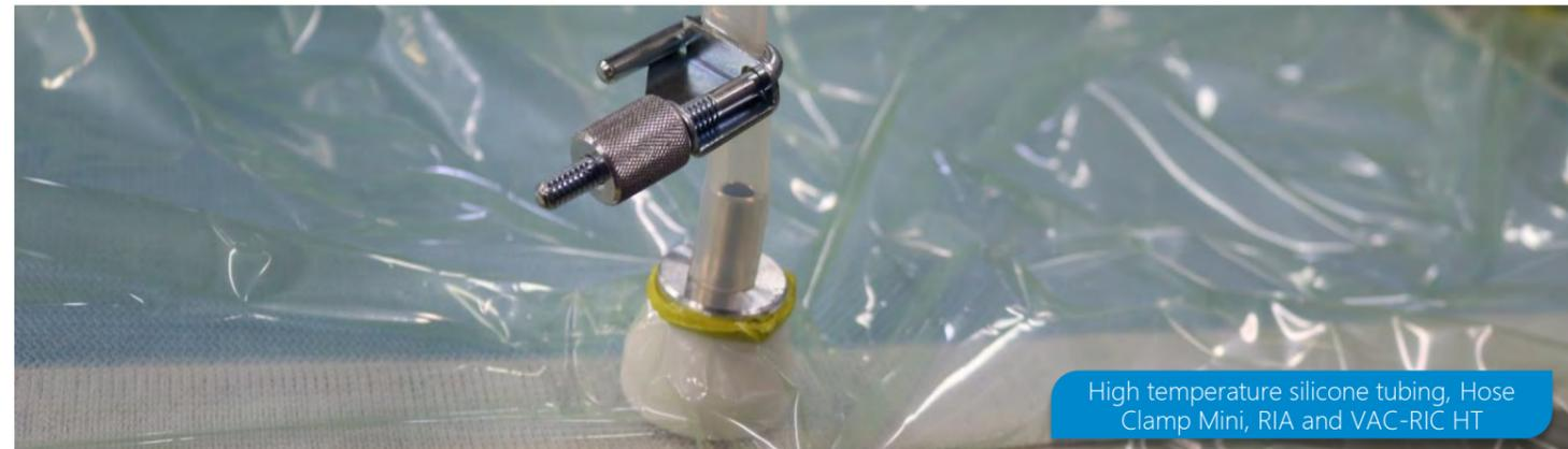
High temperature silicone tubing, Hose Clamp Mini, RIA and VAC-RIC HT
