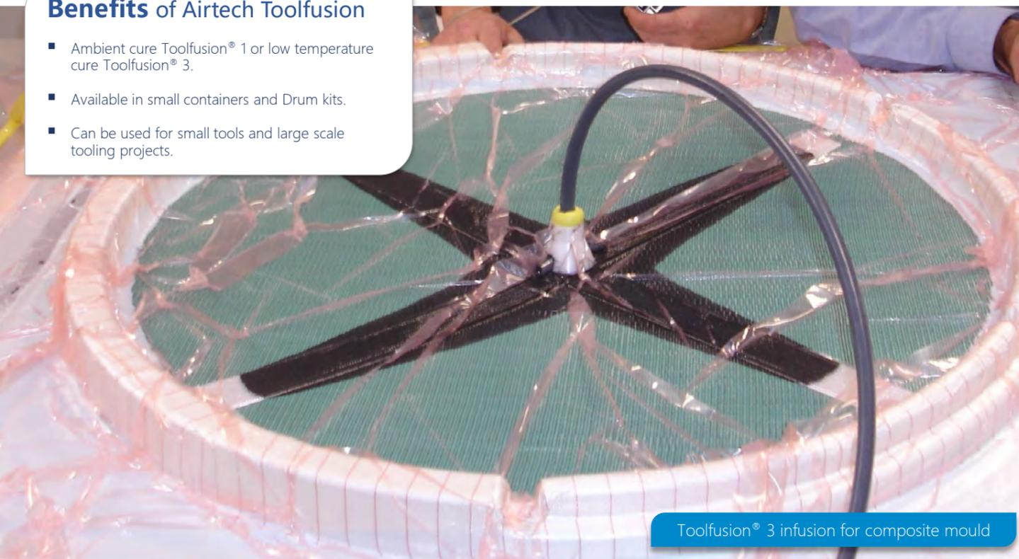
Toolfusion® 3 infusion for composite mould
