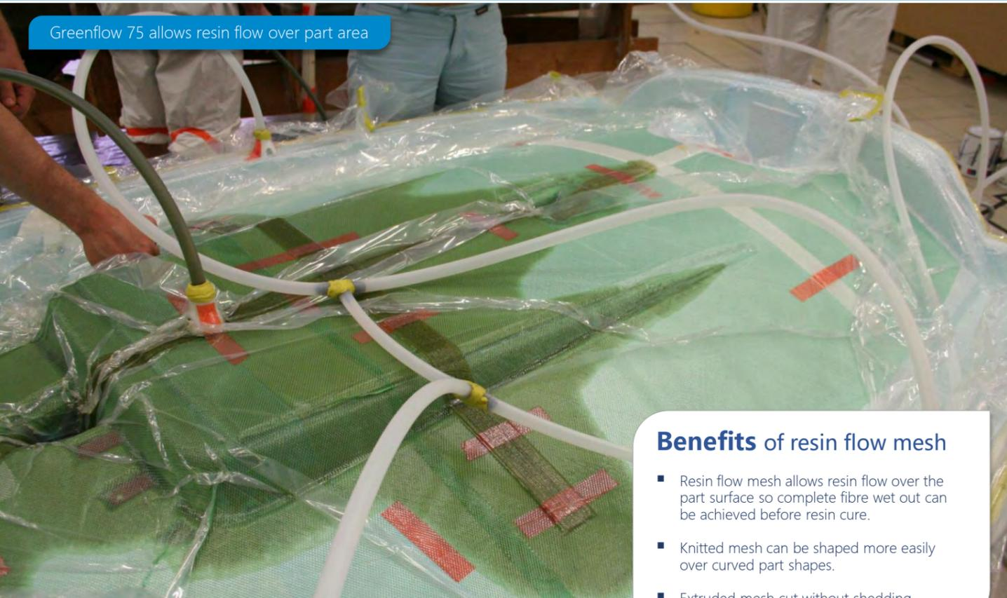
Greenflow 75 allows resin flow over part area
