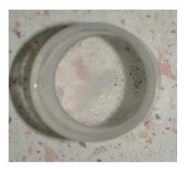
The picture of the sample after the spontaneous ignition test with oxygen
