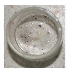
The picture of the sample after the spontaneous ignition test with oxygen
