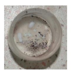
The picture of the sample after the autogenous ignition test with oxygen
