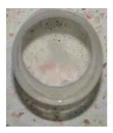
The picture of the sample after the spontaneous ignition test with oxygen
