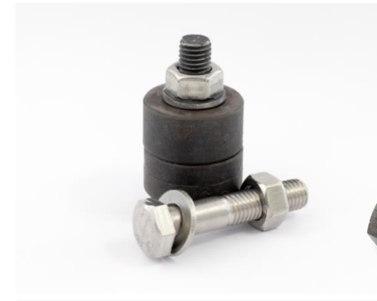
Lubricated stainless steel bolts after exposure to >500°C
