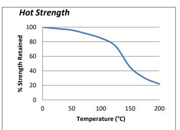
"Hot strength" shear strength tests performed on mild steel. Fully cured then conditioned to pull temperature for 30 minutes before testing.
