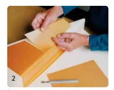
Position wax sheets onto model or tool. Use butt joints or the overlay and cut jointing technique.
