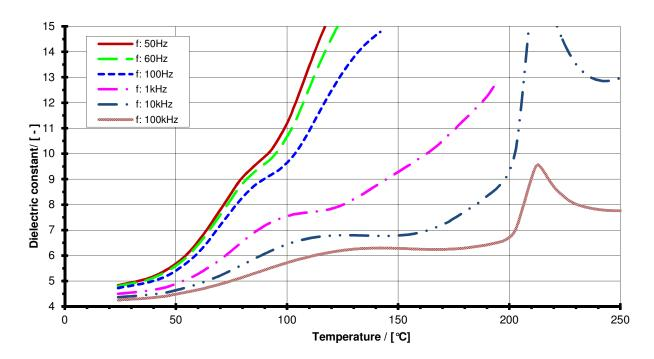
Fig. 5.1: Dielectric constant ε<sub>R</sub> vs temperature (IEC 60250)
