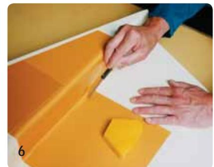
6 Repair of imperfections in joints by using Wax or Plast-Econ Modeling Clay.
