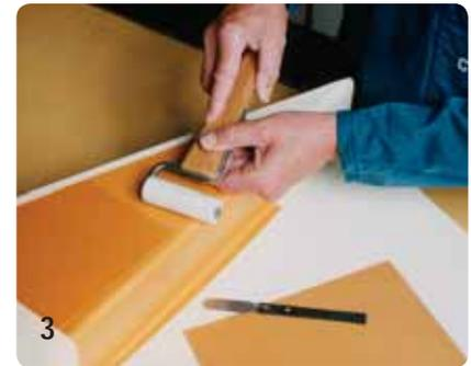
3 Roll to extrude air bubbles for a flat, even surface.
