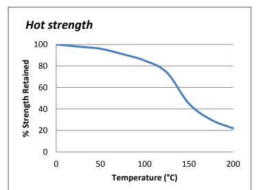
"Hot strength" shear strength tests performed on mild steel. Fully cured then conditioned to pull temperature for 30 minutes before testing. ES560 can withstand higher temperatures for brief periods (such as for paint baking and wave soldering processes) providing the joint is not unduly stressed. The minimum temperature the cured adhesive can be exposed to is -40°C (-40°F) depending on the materials being bonded.
