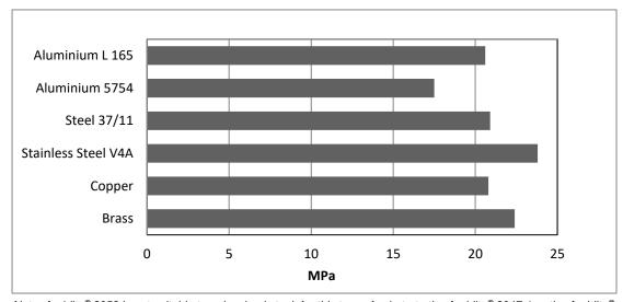
Note: Araldite® 2053 is not suitable to galvanized steel, for this type of substrate the Araldite® 2047-1 or the Araldite® 2051 may be used.
