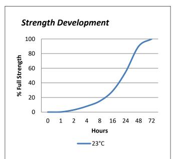
Graph shows typical strength development of bonded components at 23°C. Curing at higher or lower temperatures may affect cure speed.
