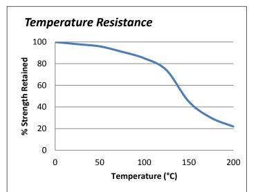
ES5681 can withstand higher temperatures for brief periods (such as for paint baking and wave soldering processes) providing the joint is not unduly stressed. The minimum temperature the cured adhesive can be exposed to is -40°C (-40°F) depending on the materials being bonded.
