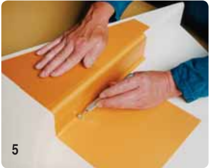
Consolidation of corners using filletting tools.
