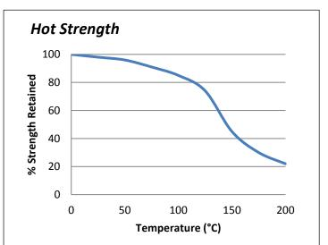
"Hot strength" shear strength tests performed on mild steel. Fully cured then conditioned to pull temperature for 30 minutes before testing. ES579 can withstand higher temperatures for brief periods (such as for paint baking and wave soldering processes) providing the joint is not unduly stressed. The minimum temperature the cured adhesive can be exposed to is -40°C (-40°F) depending on the materials being bonded.
