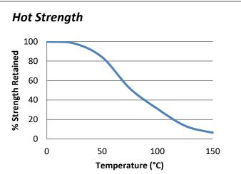
"Hot strength" shear strength tests performed on mild steel. Fully cured specimens conditioned to pull temperature for 30 minutes before testing at temperature. TA4230 can withstand higher temperatures for brief periods (such as for paint baking and wave soldering processes) providing the joint is not unduly stressed. The minimum temperature the cured adhesive can be exposed to is -40°C (-40°F) depending on the materials being bonded.
