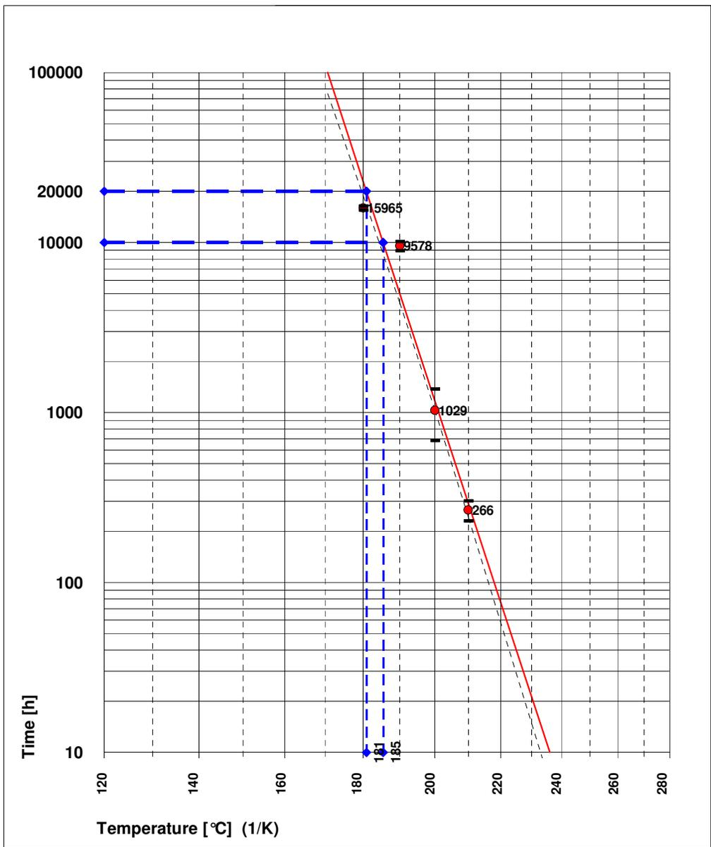
**Fig. 6.1: Thermal endurance profile (IEC 60216)**
