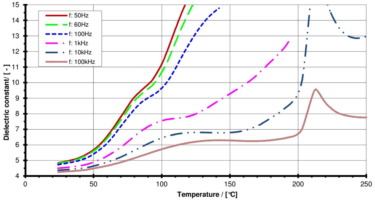
Fig. 5.1: Dielectric constant  $\epsilon_R$  vs temperature (IEC 60250)
