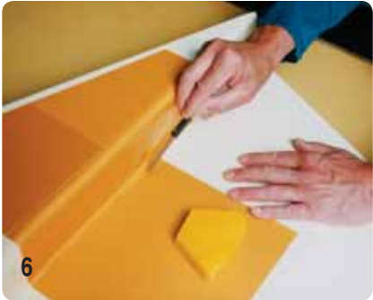
Repair of imperfections in joints by using Wax or Plast-Econ Modeling Clay.
