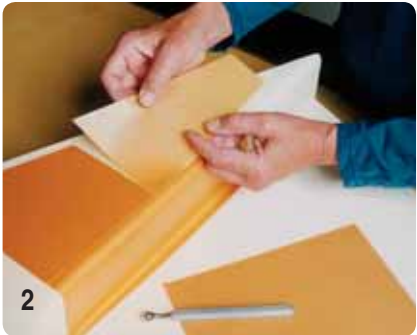
Position wax sheets onto model or tool. Use butt joints or the overlay and cut jointing technique.
