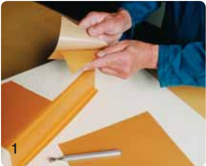
Remove the backing from the self-adhesive wax sheets or apply Sheet Wax Spray Adhesive per directions on plain sheet wax.
