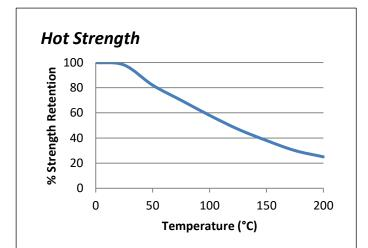
"Hot strength" shear strength tests performed on mild steel. 24hr cure at room temperature and conditioned to pull temperature for 30 minutes before testina.
