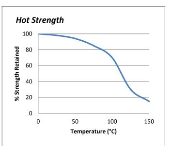
"Hot strength" shear strength tests performed on glass to mild steel. Fully cured specimens conditioned to pull temperature for 30 minutes before testing at temperature.
