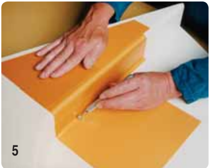
5 Consolidation of corners using filletting tools.
