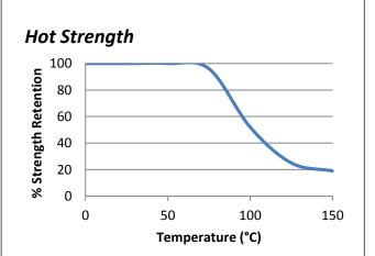
"Hot strength" shear strength tests performed on mild steel. Fully cured specimens conditioned to pull temperature for 30 minutes before testing at temperature. ET5365 can withstand higher temperatures for brief periods (such as for paint baking and wave soldering processes) providing the joint is not unduly stressed. The minimum temperature the cured adhesive can be exposed to is -40°C (-40°F) depending on the materials being bonded.
