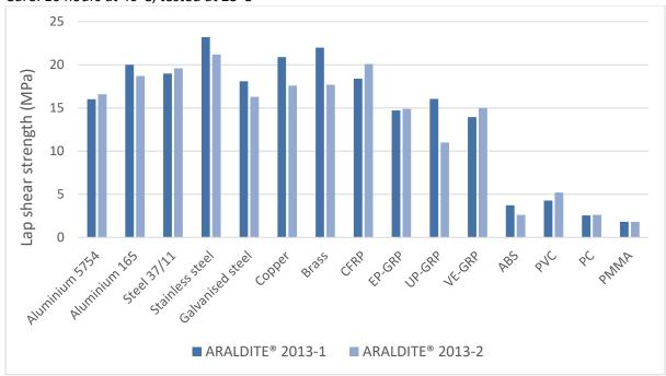
Metal substrates: sandblasted & degreased with acetone Plastic substrates: abraded & degreased with isopropanol
