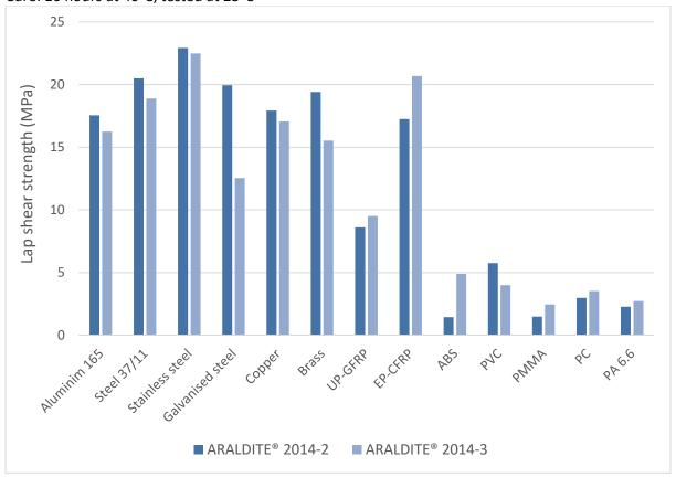
Metal substrates: sandblasted & degreased with acetone Plastic substrates: abraded & degreased with isopropanol
