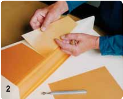
2 Position wax sheets onto model or tool. Use butt joints or the overlay and cut jointing technique.
