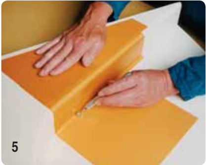
Consolidation of corners using filleting tools.
