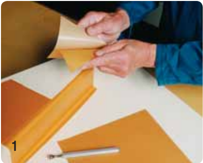
1 Remove the backing from the self-adhesive wax sheets or apply Sheet Wax Spray Adhesive per directions on plain sheet wax.
