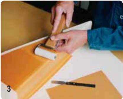
3 Roll to extrude air bubbles for a flat, even surface.
