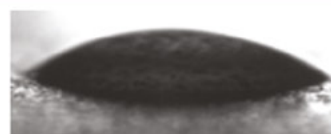
MOULEX® WD401 wettability on a mold surface WITH BOUCHEX
