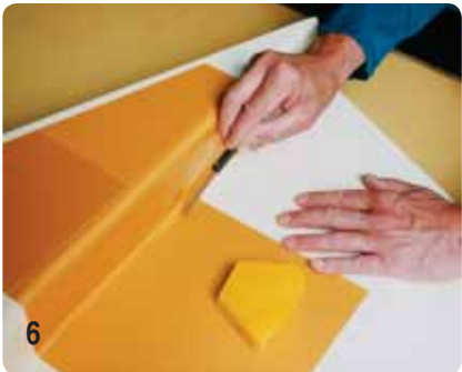
6 Repair of imperfections in joints by using Wax or Plast-Econ Modeling Clay.
